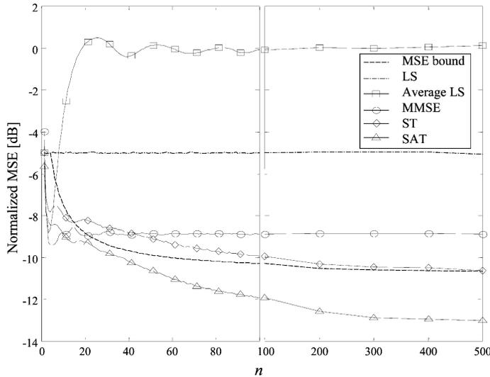
Fig. 4. Normalized  $\overline{\text{MSE}}$  versus the number of blocks  $n$  of LS (dashed lines), multiblock average of LS estimates, MMSE-FIR filtering of the LS estimates, ST, and SAT for  $f_D = 200$  Hz. Also shown as a reference is the MSE bound for ST computed in the Appendix. The left side shows the simulation results with adaptive estimation of the rank  $\hat{r}_n$  whereas for the right side the rank is set to  $\hat{r}_n = \bar{r} = 4$ .
