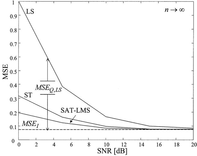
Fig. 7. *MSE* versus *SNR* for different estimators compared to the error floor set by the interpolation error.
