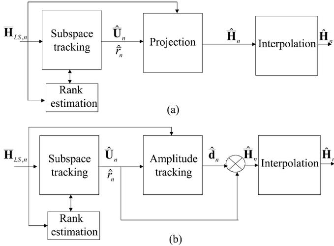
Fig. 3. Block diagrams of the (a) ST and (b) SAT algorithms.
