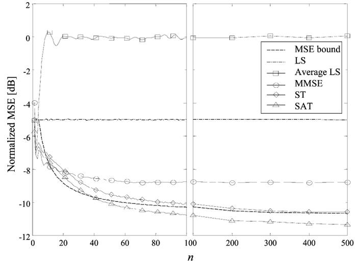
Fig. 5. Normalized  $\overline{\text{MSE}}$  versus the number of blocks  $n$  of LS (dashed lines), multiblock average of LS estimates, MMSE-FIR filtering of the LS estimates, ST, and SAT for  $f_D = 500$  Hz. Also shown as a reference is the MSE bound for ST computed in the Appendix. The left side shows the simulation results with adaptive estimation of the rank  $\hat{r}_n$  whereas for the right side, the rank is set to  $\hat{r}_n = \bar{r} = 4$ .
