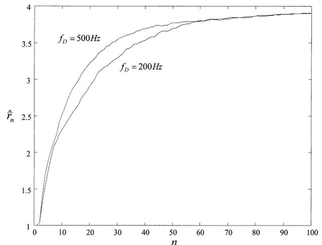
Fig. 6. Adaptive estimate of the rank  $\hat{r}_n$  for  $f_D = 200$  and  $f_D = 500$  Hz.
