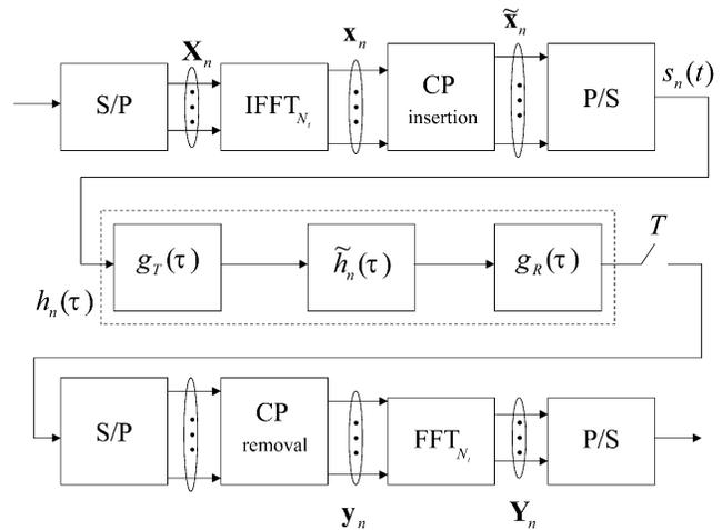
Fig. 2. Baseband model of an OFDM system.
